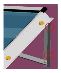
Note: For double collectors, please assemble the other collector same as Step 1 to Step 3. And keep the distance between two collectors to be 60cm at least (also need consider the length of PEX Black Pipe). As picture.
